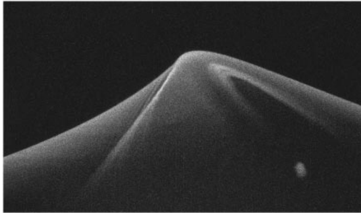
FIGURE 6. Photographs of wave crests from high-speed movie, f = 1.42 Hz A/\lambda_0 = 0.0487 . The horizontal field of view is about 111 mm. The bulge and toe are just beginning to form. t = 0 .
